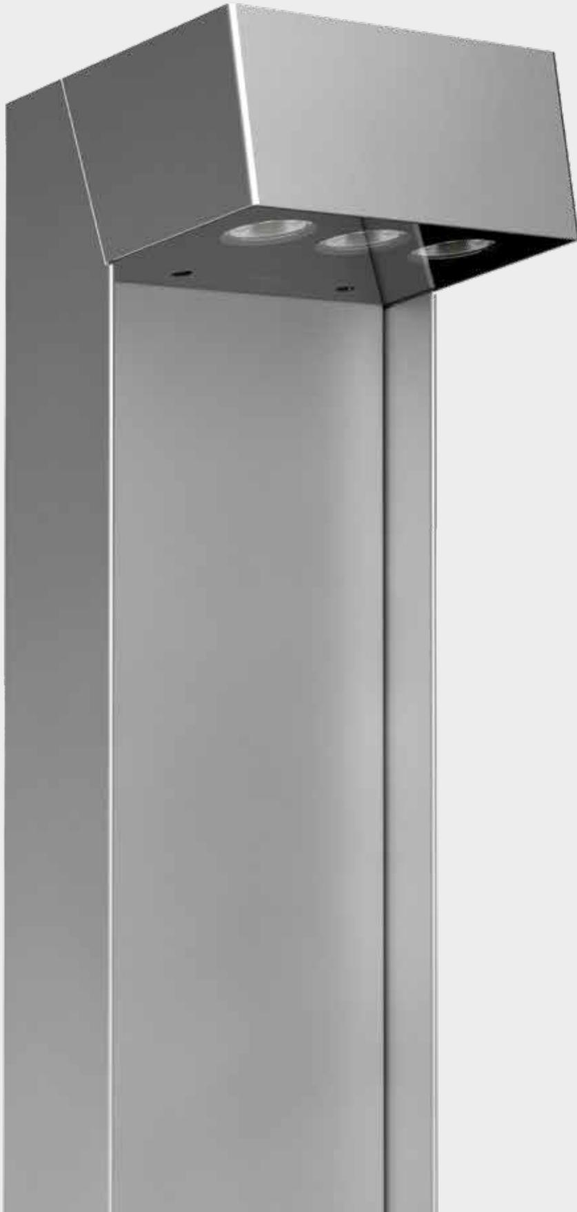
EN Bollard available in a single height of 50 cm, made of AISI 316L stainless steel. Pole head with 3 LEDs and 65° optic. Available in 2700K, 3000K and 4000K versions. Flush black silk-screened glass, extra-clear tempered 4 mm thick. Integrated power supply. Flange with anchor bolts for installation in concrete. HCT surface finish available in three variants.
