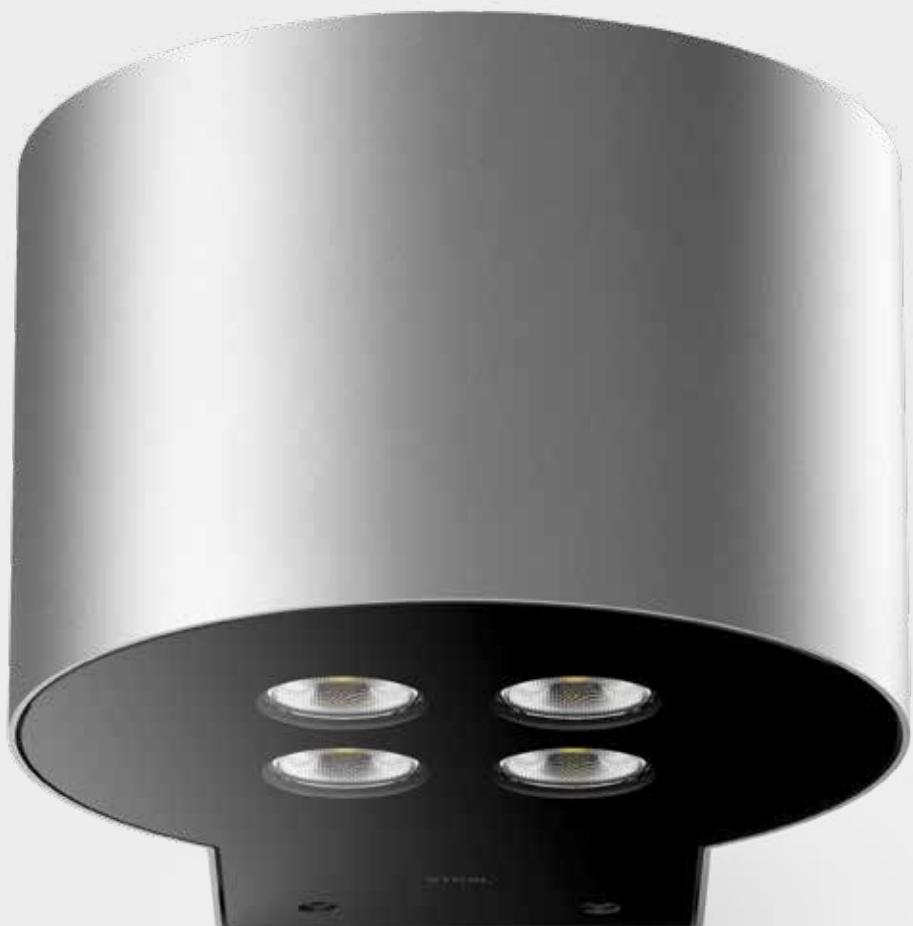
**EN** The spacer integrated with the lamp body makes the product compact. Made of AISI 316L stainless steel. Flush black silk-screened glass extra-clear tempered, 4 mm thick. Available in single and bi-emission versions in three distinct diameters for different design needs. 21°, 45° and 65° optics with color temperatures of 2700K, 3000K and 4000K. Integrated power supply. HCT surface finish available in three variants.
