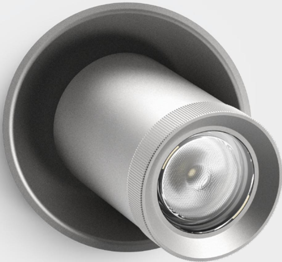
EN Closing ring with parallel lines knurling. Projector and housing base in AISI 316L stainless steel. Extra-clear tempered glass 4 mm thick. 360° rotation of the projector inside the base. GU4 lampholder for the D-50 version with remote power supply and GU10 for the D-70 version. HCT surface finish available in three variants. Installation on the floor, wall, and ceiling through apposite bracket.
