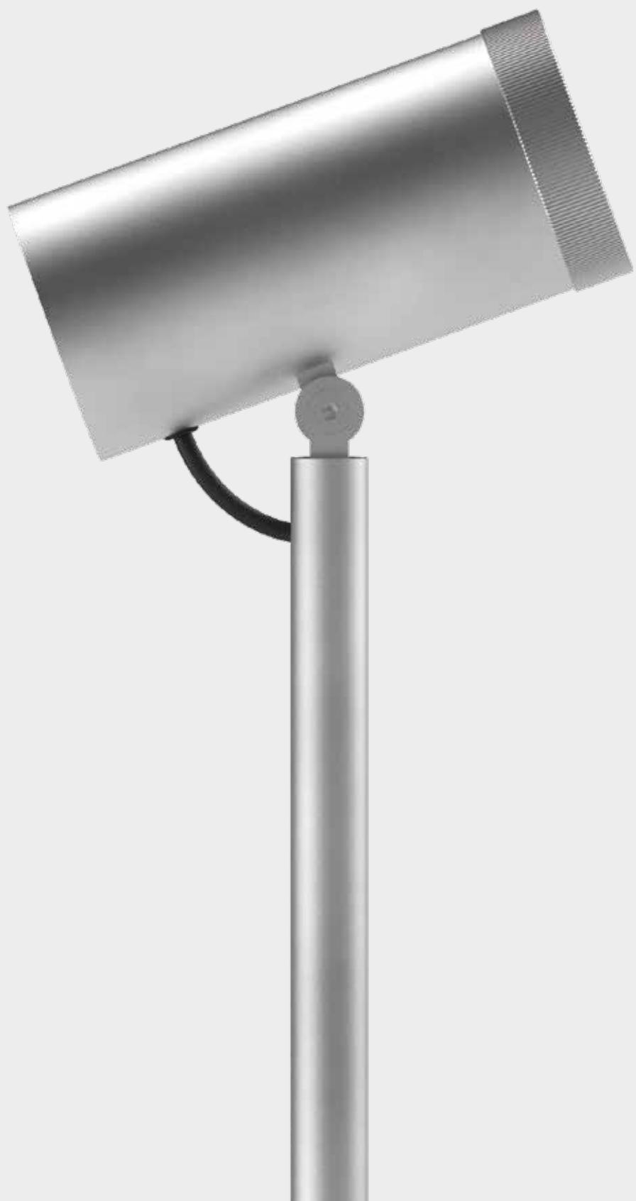
**EN** Projector with locking ring with parallel lines knurling. Spike and projector in AISI 316L stainless steel. Extra-clear tempered glass 4 mm thick. Power cable inserted inside the spike for protection against cuts and accidental damage. Head axial rotation of 180°. GU4 lampholder for D-50 version with remote power supply and GU10 for D-70 version. HCT surface finish available in three variants.
