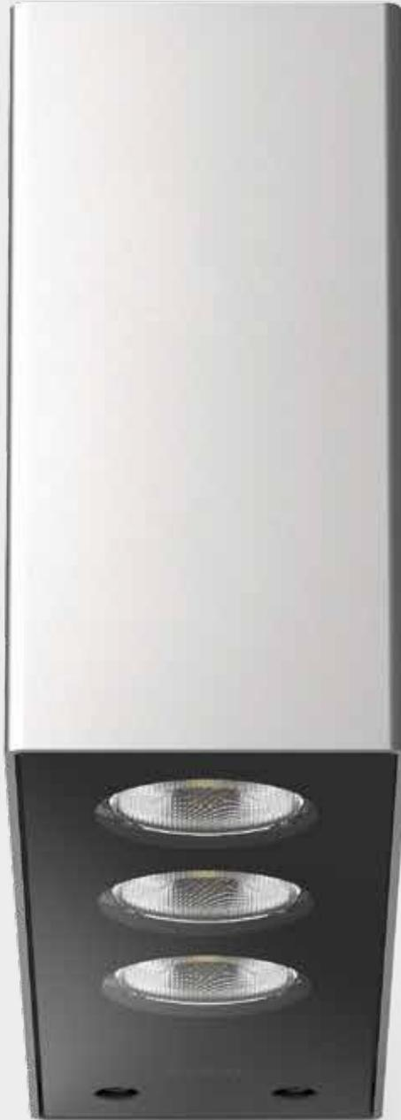
EN The spacer integrated with the lamp body makes the product compact. Made of AISI 316L stainless steel. Flush black silk-screened glass extra-clear tempered, 4 mm thick. Mono and bi-emission versions with one, two or three LEDs for different design needs. 21°, 45° and 65° optics at 2700K, 3000K and 4000K. Integrated power supply. HCT surface finish available in three variants.
