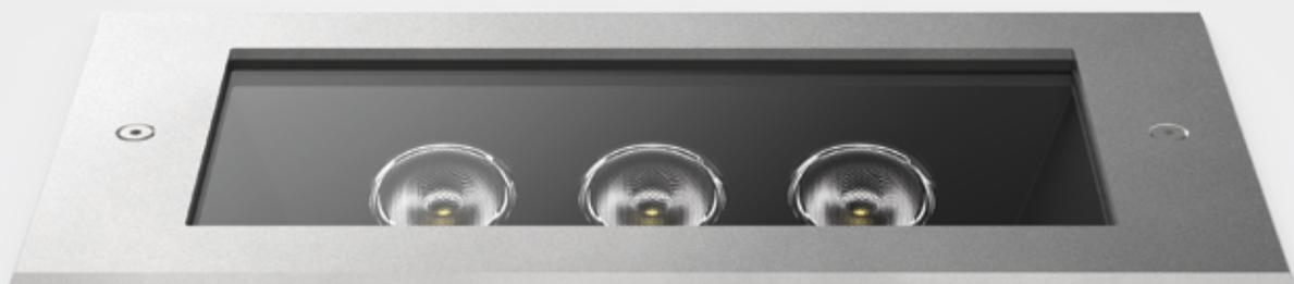
**EN** Frame and lamp body in stainless steel, including the part recessed in the ground. Stainless steel fixing screws with color matched to the finish. Horizontal or vertical asymmetrical reflector. Optics from 21°, 45° and 65° at 2700K, 3000K and 4000K. Installation in the ground and/or on the floor through polyethylene outer casing. 8mm extra-clear tempered glass. Integrated power supply. HCT surface finish available in three variants.
